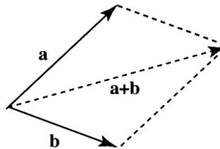
**Fig. 3.11 The parallelogram method of addition**
