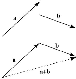
**Fig. 3.10 The triangle method of addition**
