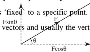
The vertical component when used with forces is usually drawn from the same position as the original force as indicated in figure 3.4.
