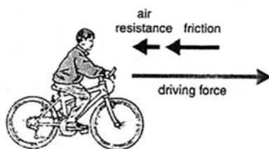
**Fig. 3.1 Forces in a horizontal direction**
